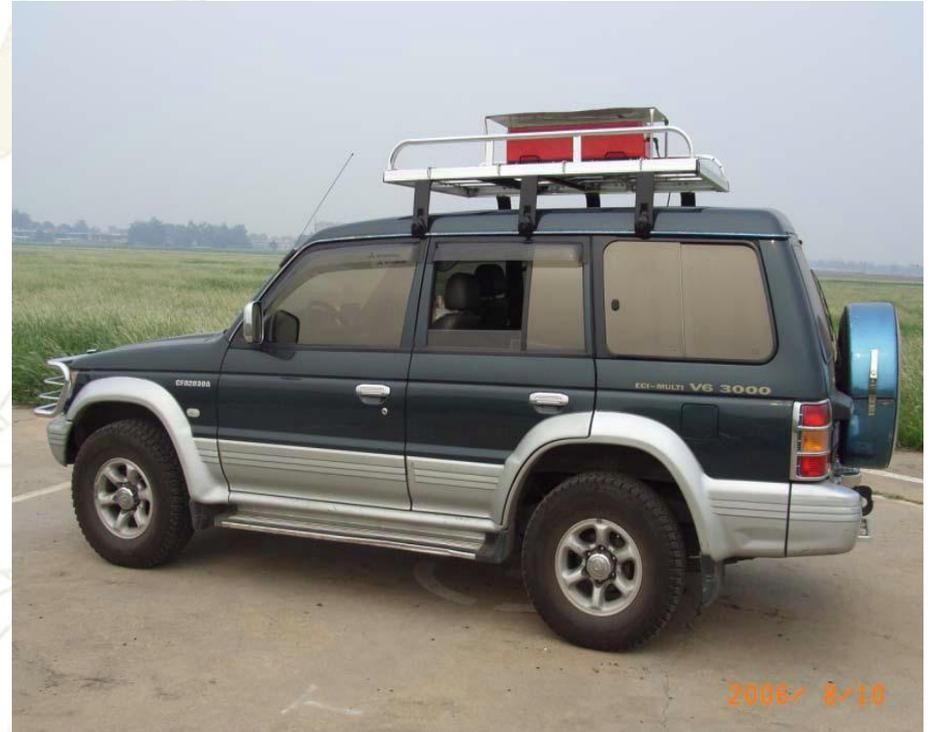
The CGS system was installed in jeep, with large volume(4L), GR460, NaI(Tl) detector.
